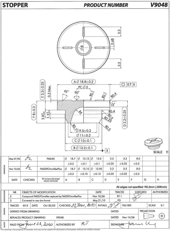
Dimensions without tolerance indication correspond to DIN-ISO 3302 Class M3. Cut or punched edges can be slightly conical, excentric and/or variable.
